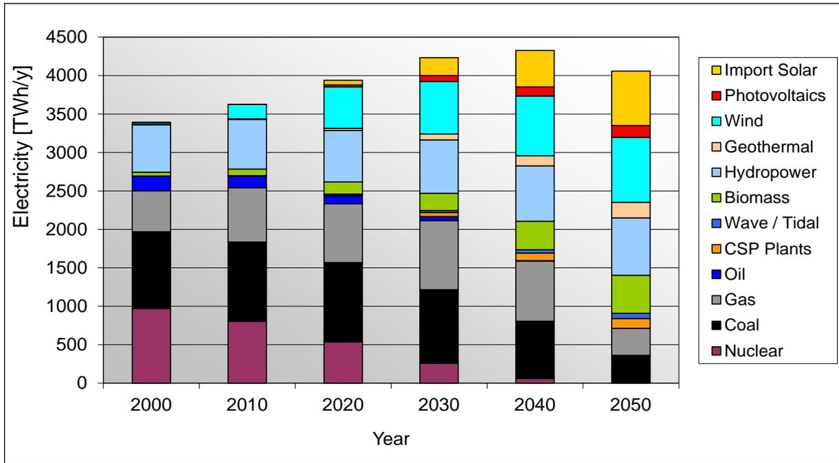
**Figure 1:** Annual electricity supply according to the original scenario TRANS-CSP (2006) with 80% renewable share characterized by stagnating power consumption, nuclear phase-out and solar electricity imports from North Africa to Europe.
